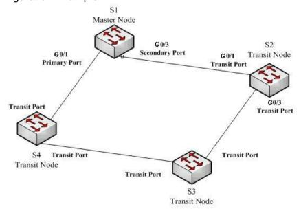
Figure 2.1 Fast Ethernet Ring Protection Configuration Example
